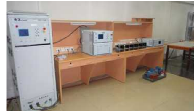
AC source Surge Noise coupler EFT
