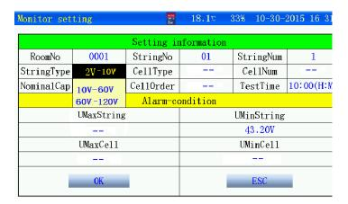
Online monitoring for battery string: when the battery pack is under the state of online discharge, uniform charge and floating charge, perform real-time online monitoring for all cells. The monitoring includes string voltage, cell voltage, charge/discharge current, monitoring time of battery string, charge/discharge capacity of battery string and etc.
