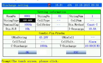
Perform discharge of constant current taking advantage of intellectualized dummy load after the battery pack is removed from system, set up the parameters of "discharge current", "discharge time", "discharge capacity", "final protective voltage of whole pack" and" final protective voltage of cell", and the tester could carry out discharge function automatically, display discharge current, battery discharged capacity, the whole pack voltage, cell voltage, discharge time and etc at real time;
